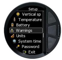
When you press middle button for longer time, you will get into setup menu. Press upper and lower button to move focus. Quickly press middle button to enter submenu. Long press middle button to exit submenu or select Exit option in menu.
