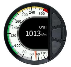
QNH display will be automatically closed few seconds after last button was pressed.
