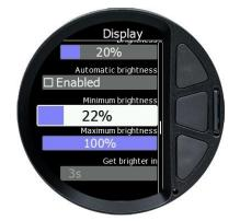
Press middle button to enter edit mode. Slider background colour will change to white. Use upper and lower button to increase or decrease value. Long press will make a bigger increase or decrease. Confirm selection with short press on middle button. Long press middle button to cancel selection and exit without changes.
