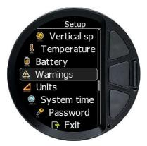
When you press middle button for longer time, you will get into setup menu. Press upper and lower button to move focus. Quickly press middle button to enter submenu. Long press middle button to exit submenu or select Exit option in menu.
