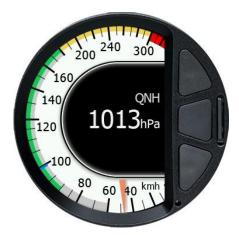
QNH display will be automatically closed few seconds after last button was pressed.
