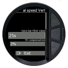
TE compensation is used mainly for gliders in order to show total energy change rather than vertical speed. Set to 100%, if you want to have compensated vertical speed indication or leave on 0 to have non-compensated vertical speed.
