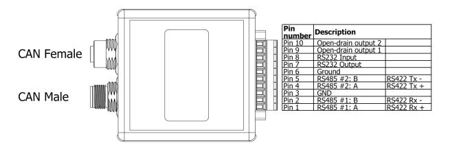
If CAN bridge is connected to S-vario, additionally is delivered M12 to DB9 (CAN BUS cable)
