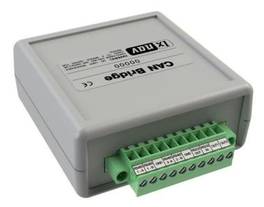
LXNAV CAN bridge is connected to the CAN bus through a male or female M12 connector. Power is derived from CAN bus and no external power is needed. The device does not contain a CAN terminator.
