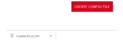
To load this file into FlarmBat, copy it on micro SD card, insert it into FlarmBat and switch it ON. File will be automatically loaded into device.
