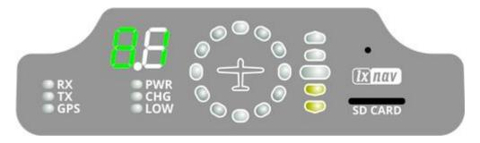
On picture below is code 81, which means No Obstacles.
