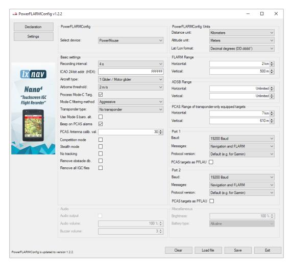
Here you can set all settings for your FlarmBat device. File will be saved as flarmcfg.txt file, which you should save on the micro SD card. To load this file into FlarmBat, insert micro SD card in FlarmBat and switch it ON. File will be automatically loaded into device. You can configure existing flarmcfg.txt, which is present on micro SD card.
