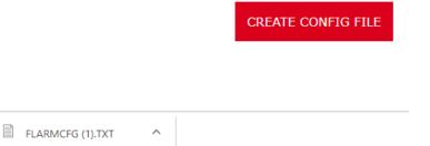
To load this file into FlarmBat, copy it on micro SD card, insert it into FlarmBat and switch it ON. File will be automatically loaded into device.
