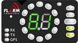
On picture below is code 81, which means No Obstacles.
