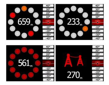
The screen indicates relative position of threat. In the first image two gliders are approaching from left side at the same altitude and one from back right, the second screen one glider is approaching from right side (4'o clock), third screen is an example of undirected warning (AC mode). Middle number shows horizontal distance to the target, last picture indicates obstacle warning.
