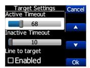
With **Edit** you can activate slider control, then **up/down** buttons you can select the preferred value and confirm it with the **Ok** push button.
