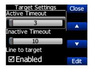
In FlarmView57 up and down means rotating left and right the knob, Short press is same as **Edit**, long push is same as **Close**
