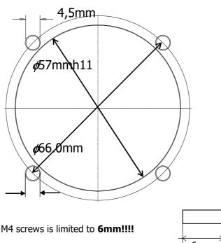
The length of the M4 screws is limited to 6mm!!!!
