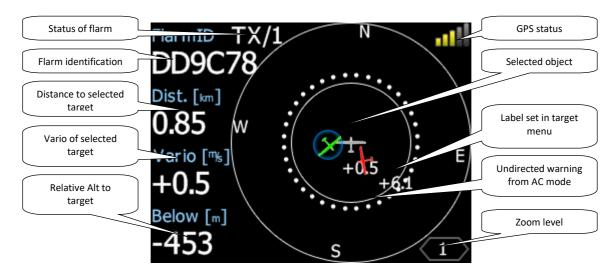
**Status of Flarm** TX/2, means, that flarm device transmits data, 2 means, that Flarm receives data from two Flarm devices.
