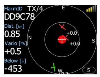
All targets are displayed as a glider symbols. User can change that symbol to another type. It's also possible to change object color, depending on relative altitude to us. All received targets (Flarm or PCAS) are marked with same type of symbol except undirected targets, for which we don't know from which direction they are comming from. Flarm targets can be separated only by their ID.
