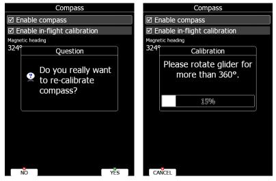
Keep rotating glider until progress reaches 100%. Calibration will automatically exit and compass calibration is finished. Check compass directions afterwards, they should be within +/-2 degrees. Press PTT on radio to see if there is any deviation in magnetic heading.
