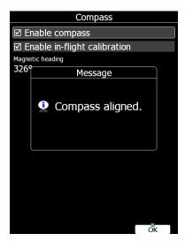
Press **CALIB** button to start calibration of compass on the ground. Calibration process I very straightforward. Make sure glider fuselage is levelled (use tail dolly), wings are levelled and canopy is closed with pilot inside. Switch on all the avionics, which is normally switched on while flying. Confirm calibration of compass to start calibration process. Assistant on the wing should slowly rotate glider with wings levelled.
