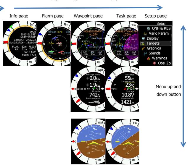
To enter a task, select task page. A short press of the bottom rotary knob activates the quick access menu. In addition to MacCready, Ballast and Bugs you can Start, or Edit a task. If the Task is started you can restart or go to the next waypoint. You can also change the Navboxes through this menu.
