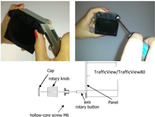
Remove the two rotary knob caps with a knife or a flat screwdriver, then hold each knob and unscrew it. Remove the remaining two screws and the two M6 threaded nuts. Install the knobs and the panel there is sufficient space so that the button can be pushed.
