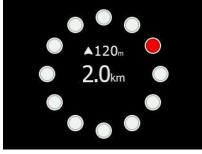
If "modern view" is chosen, warnings will be displayed as a 3D visualisation of the approaching threat. This is for the highest alarm level (level 3) and indicates that impact is 0-8 second (s) away. The example picture shows (us) an airplane approaching (us) you from front left (11 o'clock) 40m below us. This screen will only be displayed if the airplane is approaching head-on (from the front).
