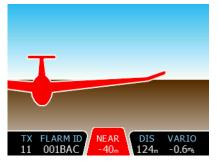
Obstacle warning, the upper number indicates the distance to object. The smaller lower number indicates the relative altitude.
