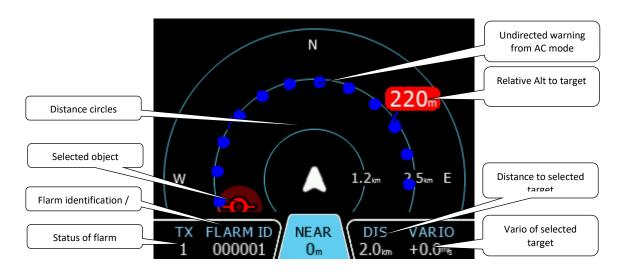
**Relative altitude** shows the vertical distance to the target. If there is a – symbol in front of the target, the target is below you (e.g. -200), if not it is above you (e.g. 200m).
