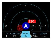
Targets are displayed as a series of symbols, as shown in the table below. It's also possible to change the object colour, depending on the relative altitude to the airplane. You can do this by going to Setup-> Graphic-> Traffic. All received targets (Flarm or PCAS) are marked with the same type of symbol except undirected targets, for which we don't know what direction they are travelling to. Flarm targets can be separated only by their ID.
