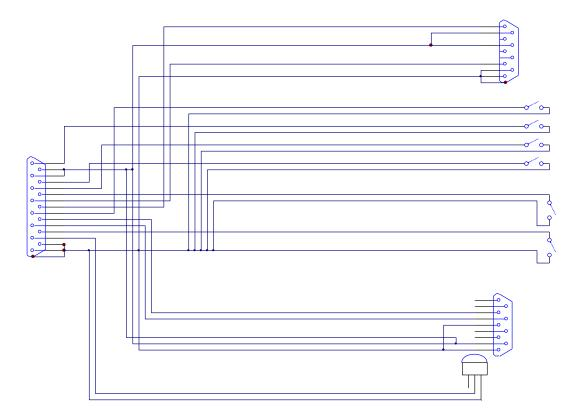
V5 has four additional inputs comparing to the old vario systems. Those inputs can be connected to Eg. Gear, Airbrake switches, which can be set in setup-hardware-variometer.
