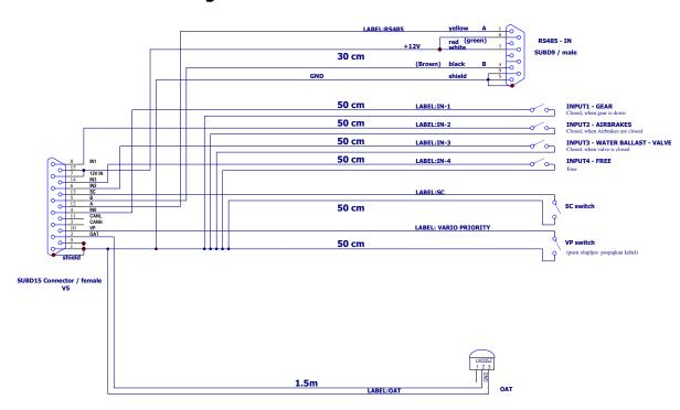
V8X has four inputs. These inputs can be connected to Eg. Gear, Airbrake switches and can be set in setup-hardware-variometer.
