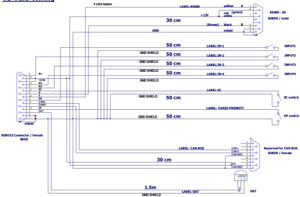
V9 has four additional inputs comparing to the old vario systems. Those inputs can be connected to Eg. Gear, Airbrake switches, which can be set in setup-hardware-variometer.
