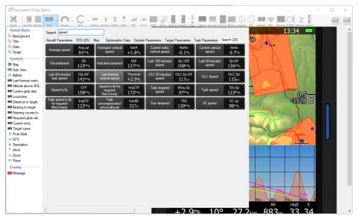
Data symbols are grouped in seven groups: aircraft parameters, outside parameters, target parameters, task parameters, optimization data, FES/JDU and misc tab. More details about the data symbols of each tab are available in chapter 3.2.2.
