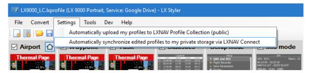
When you open a file with enabled synchronization, LX Styler will check if the remote file has changed, and if the file you just opened has been modified outside of LX Styler. In case only one of the files was modified, the one that was modified will be loaded, if both we're modified you will be prompted which one you would like to load.
