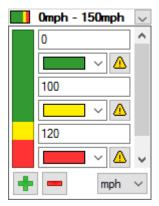
You can add a new range, or remove it with the "+ and — buttons" on the bottom left. After pressing the button, hoover over the tape on the left side, and click on the range to remove it, or split it in two. If you press "add new", you can also select the up or down arrow to add a new range on the top, or on the bottom of the scale. On the bottom right side, it is possible to select the unit in which the values will be written.
