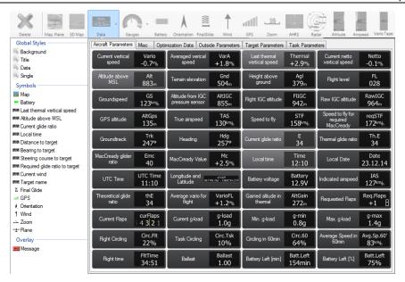
Data symbols are grouped in seven logical groups: aircraft parameters, outside parameters, target parameters, task parameters, optimization data, FES/JDU and misc tab. Specific symbols will be depicted in the next chapter.
