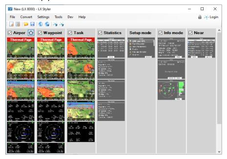
The main window consists of a menu, a toolbar and a general view, where all the seven navigational modes are shown, namely airport mode, waypoint mode, task mode, statistics mode, setup mode, info mode, and near mode.
