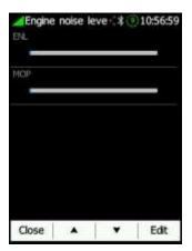
This page is just for monitoring the Environmental Noise Level ENL. MOP (means of propulsion) is provided to detect noises produced from JET engines.
