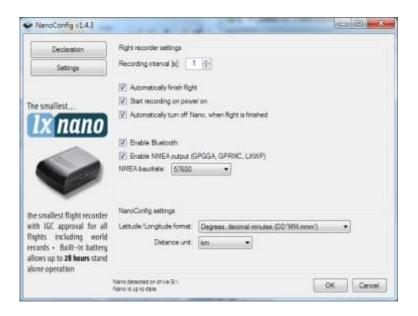
Parameters for the NANO<sup>4</sup> include the recording interval, a NMEA output and a Bluetooth enable setting.
