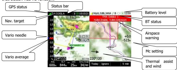
At the bottom of the map screen there is navbox row with 4 navboxes. By swiping the navbox row you can configure up to 12 different navboxes for each page mode. With a long press on the nav box the user can select many navbox options.
