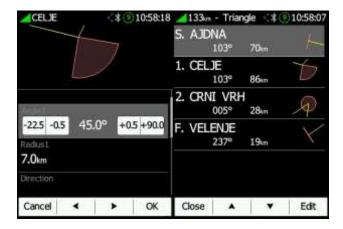
When using parameters in the zone dialogue, it is possible to describe all types of observation zones. **Angle12** defines the orientation of the observation zone. Available values for **Direction** are:
