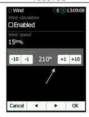
The NANO<sup>4</sup> will automatically calculate and display current wind information. Alternatively, when this option is disabled, you can enter wind data yourself. You can do this by manually adjusting the wind speed and direction or by simply dragging the arrow over the bottom part of the screen.
