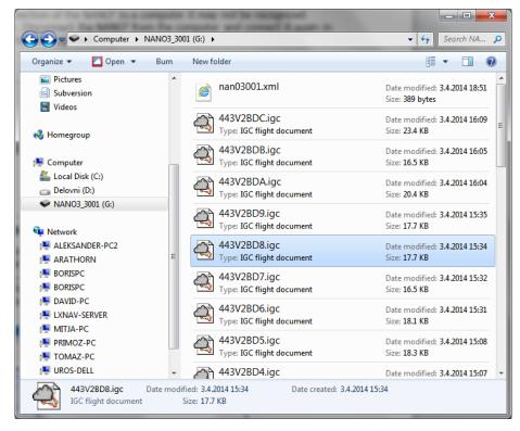
Flights are stored on files with the IGC standard filename. If you find it difficult to decode this standard, we recommended that you switch to detailed view to see the date of the file. In the detailed view the file date and time shows the landing time of the glider.
