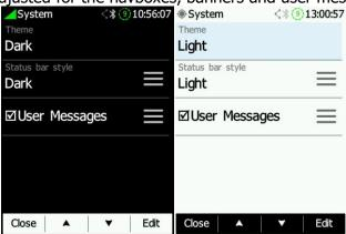
By clicking on the "hamburger" menu of the **Status bar style** you can switch between two battery status styles **Standard** and **With time** (shows how many hours/minutes is left), adjust status bar text colour and enable the seconds on time display.
