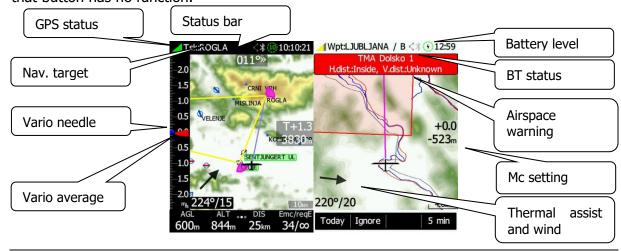
At the bottom of the map screen there is navbox row with 4 navboxes. By swiping the navbox row you can configure up to 12 different navboxes for each page mode. With a long press on the nav box the user can select many navbox options.
