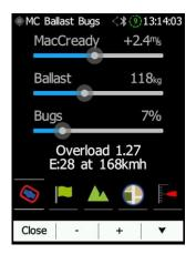
On this screen MacCready, Ballast and Bugs and map shortcuts can be adjusted. At the same time a calculated final glide and speed are displayed on the lower part of the screen.
