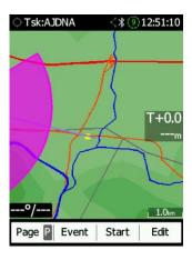
The middle buttons help with target selection by cycling through available targets. The right button has an EDIT /SELECT or EVENT function, where you can edit/view the currently selected target.
