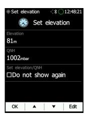
After clicking "**OK**" or waiting 30 seconds instrument will proceed to the Flight info page. The instrument is now ready to use. In the left upper corner the GPS status is displayed. The
