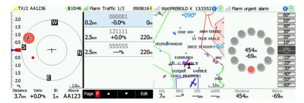
PCAS alerts on the map are represented as a dotted circle with a relative altitude; the PCAS warning is represented by lights on the clock in red or orange.
