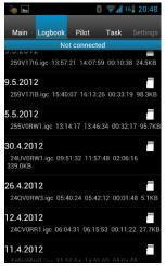
After the downloading of the logbook data is finished a short press on the desired flight will start the download process. If the flight size is large, the download may take more than one minute. Flights are downloaded into the NanoConfig folder. With a longer push on the flight one can share the downloaded flight with other applications installed on a smart phone (Gmail, SeeYou, OLC (not available), Google Docs, Facebook).
