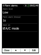
The **Flarm timeout** defines the time when the user ceases to see a FLARM warning after dismissing the FLARM warning of a FLARM object. Alert on A/C mode enables or disables whether an alarm is set off by A/C mode transponders whose location is unknown and whose distance is only approximated.
