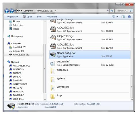
In the root folder you will find the flights created by the NANO<sup>4</sup> together with the NanoConfig program. The NanoConfig program will run only on Microsoft Windows operating systems. Double click to run it.
