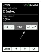
The NANO<sup>4</sup> will automatically calculate and display current wind information. Alternatively, when this option is disabled, you can enter wind data yourself. You can do this by manually adjusting the wind speed and direction or by simply dragging the arrow over the bottom part of the screen.
