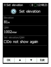
After clicking "**OK**" or waiting 30 seconds instrument will proceed to the Flight info page. The instrument is now ready to use. In the left upper corner the GPS status is displayed. The
