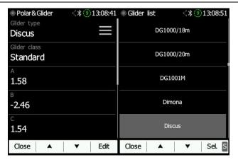
You can modify the polar by changing coefficients **a**, **b** and **c**. A polar is defined as a quadratic equation with the parameters a, b, and c.
