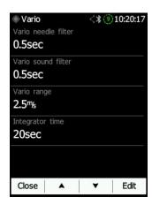
A higher number for the vario filters means a more damped vario signal. Range is the overall scale of the vario type with its maximum and minimum value. With longer integrator times the vario calculates average over the longer period.
