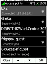
Select the Wi-Fi you wish to connect to and a new menu will open where you can type in the password and enable or disable DHCP.
