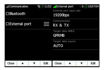
In the communication menu you can enable or disable the **Bluetooth** device, enable or disable the **NMEA output** on the **external** USB port and define the **baud rate** for the external serial interface.
