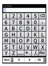
Pushing the **next** button will move the cursor to the right. A longer push on **next(P)**, will move cursor left. At the last character position pushing the button will confirm the edited value; a long press **OK(C)** will cancel editing and exit that control. If a longer push is available, part of the button label will be shown red. For example, on the above a longer push on the left button **next(P)** has a back function. A longer push on the right button has the Cancel function.
