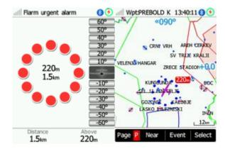
A FLARM warning can be dismissed with a short press of any button. A dismiss time can be configured in setup.
