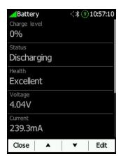
Voltage is typically between 3,5V and 4,2V. Current depends on the power consumption (LCD brightness, BT, Wi-Fi) and the voltage of battery.
