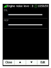
This page is just for monitoring the Environmental Noise Level ENL. MOP (means of propulsion) is provided to detect noises produced from JET engines.
