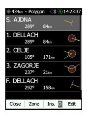
A Task can be entered in a very simple way. In the task page one can press the **edit** button. Using the up or down button one can highlight an existing waypoint or an empty space and then set a new waypoint. By pressing the **Ins**. (insert) button one can start browsing through all the waypoints in the selected CUP file.
