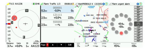
PCAS alerts on the map are represented as a dotted circle with a relative altitude; the PCAS warning is represented by lights on the clock in red or orange.
