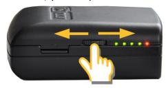
Press it and NANO flight recorder will power on. Press or move the rocker button for a long time and the NANO flight recorder will switch off. When flying press or move the button for a short time and a pilot-initiated event will be recorded and the flight recorder will then log 30 fixes with a recording rate of one per second.
