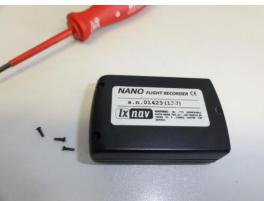
Open the cover and remove the battery:
