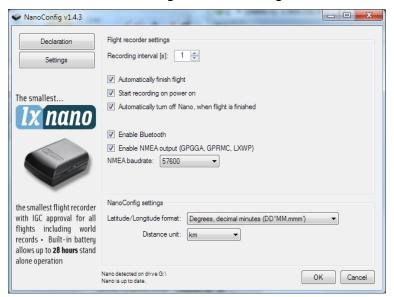
Parameters for the NANO include recording interval, NMEA output and Bluetooth enable settings.
