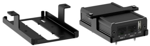
When installing PowerMouse mount first firmly mount the bottom part (left) with screws that came with the product. Then place PowerMouse into the mount and place the top bar over it as seen on picture above (right). Secure it with two screws.
