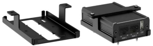
When installing PowerMouse mount first firmly mount the bottom part (left) with screws that came with the product. Then place PowerMouse into the mount and place the top bar over it as seen on picture above (right). Secure it with two screws.
