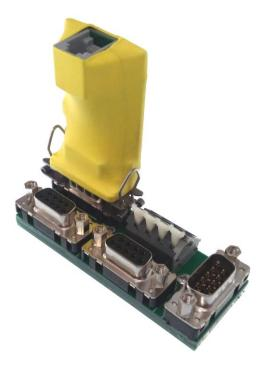
On the back side of the Bridge is a RJ12 connector with RS485 output for Trig radio or transponder. 12 V output from bridge can be only used for powering up small devices, do not power radio over this pin, it cannot supply such load. You can burn bridge or maybe even main instrument over which is powered.
